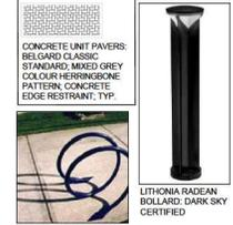
CONCRETE UNIT PAVERS: BELGARD CLASSIC STANDARD MIXED GREY COLOUR HERRINGBONE PATTERN. CONCRETE EDGE RESTRAINT, TYP.
