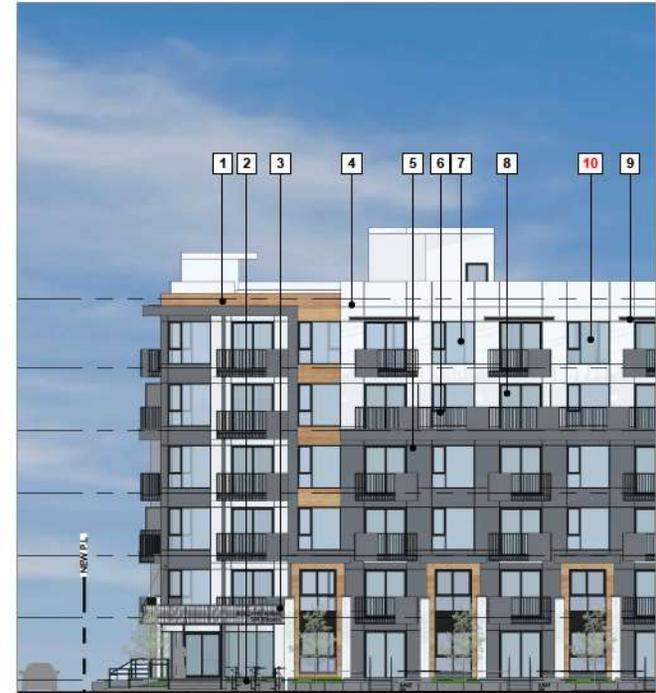
\* NOTE: All fiber cement panels trims/recess, reveals, reglets, etc. must be colored matching to the panels they are attached to.
