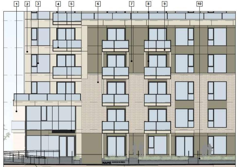
\* NOTE: All fiber cement panels trims/recess, reveals, reglets, etc. must be colored matching to the panels they are attached to.
