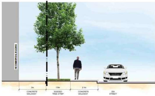
S2 SECTION THROUGH EAST PEDESTRIAN CORRIDOR 1:50
