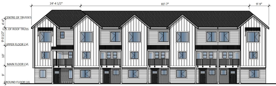
1 FRONT/EAST ELEVATION Scale: 1/16"=1'-0"
