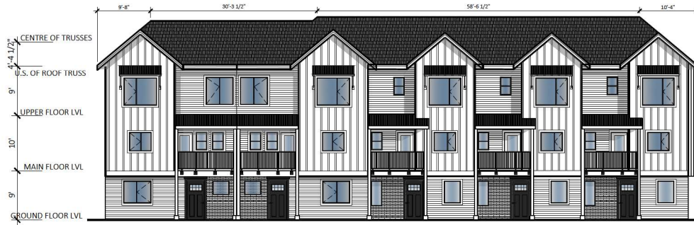
1 REAR/WEST ELEVATION Scale: 1/16"=1'-0"
