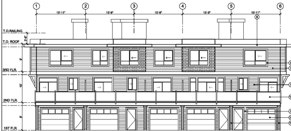
SOUTH (REAR) ELEVATION - BLOCK 1
