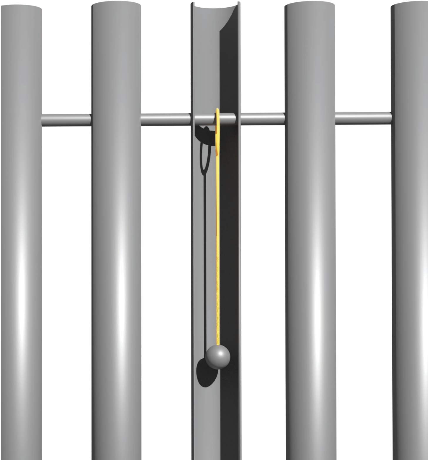
Cross section of single pipe xylophone, showing the hanging inner mallet.
