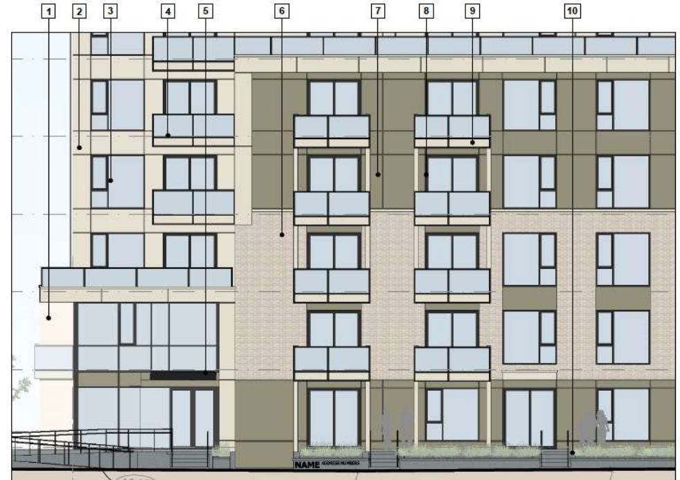
4 - Aluminium Railing with Safety Glass Clear and Translucent Color to Match: Benjamin Moore Black Ink 2127-20
