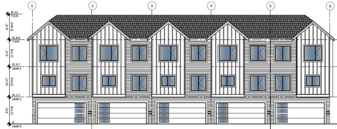
1 BACK ELEVATION Scale: 3/32"=1'-0"
