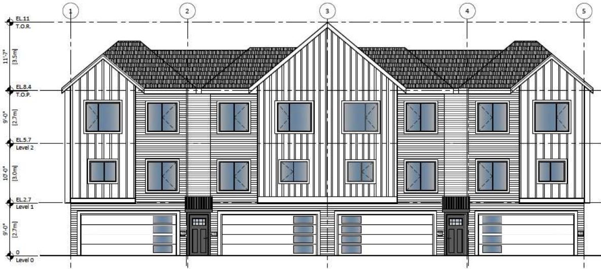
1 BACK ELEVATION Scale: 3/32"=1'-0"
