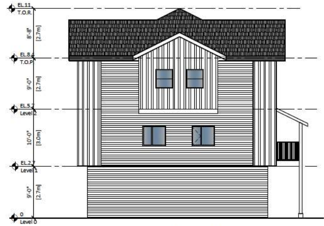
3 RIGHT ELEVATION Scale: 3/32"=1'-0"
