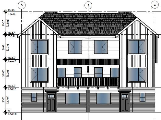
2 FRONT ELEVATION Scale: 3/32"=1'-0"
