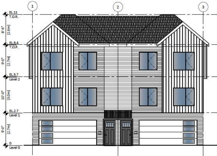
1 BACK ELEVATION Scale: 3/32"=1'-0"
