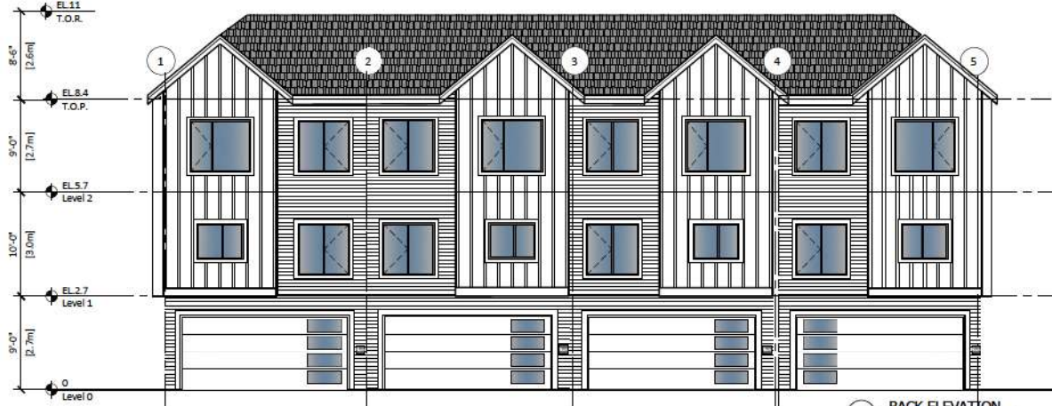
1 BACK ELEVATION Scale: 3/32"=1'-0"
