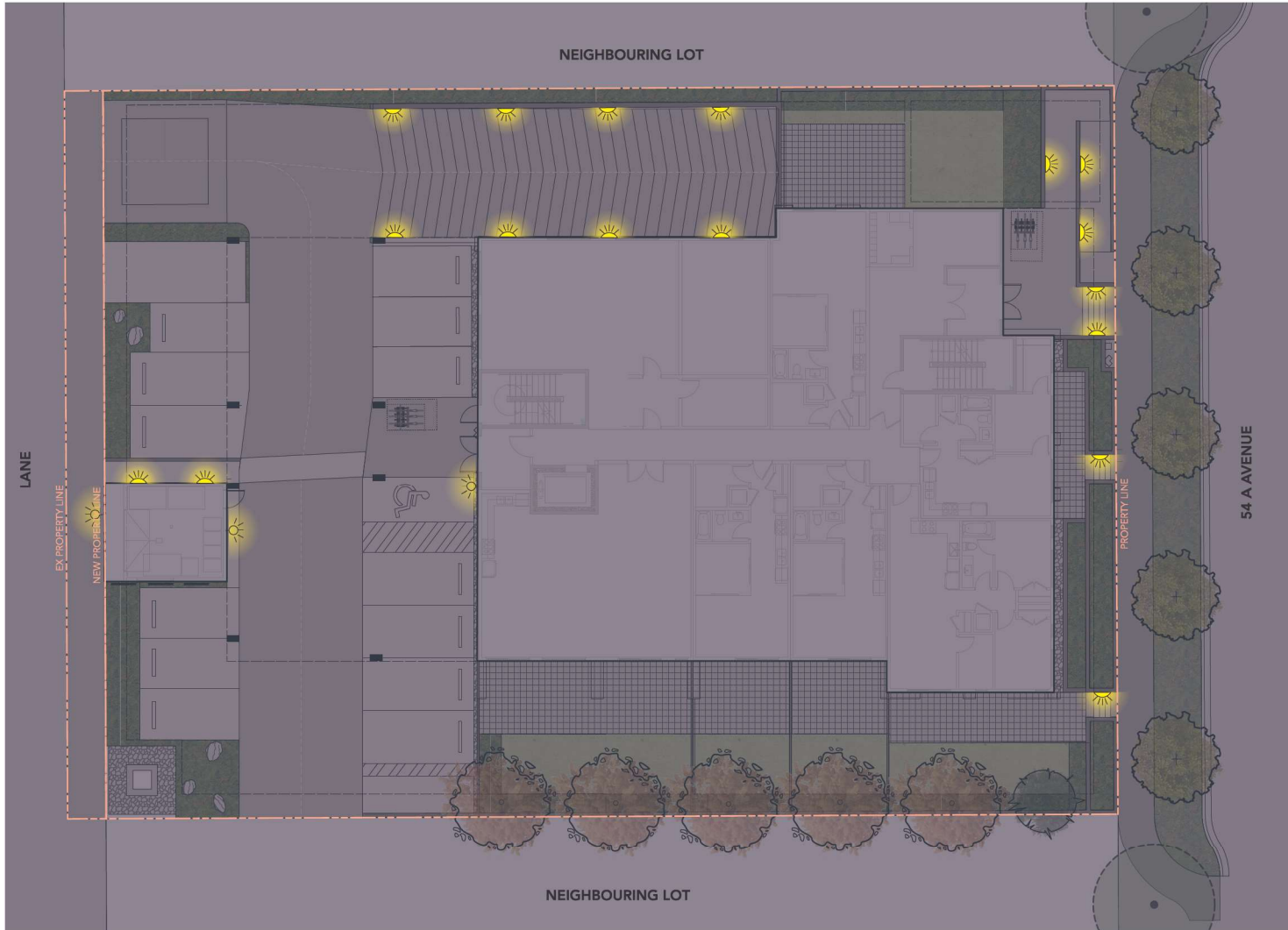
WALL DOWN LIGHT MP LIGHTING MODEL L721 4" DIAMETER, 6W LED MATTE ANODIZED ALUMINUM
