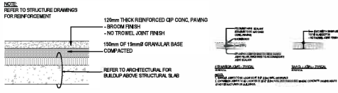
2 C.I.P. CONCRETE PAVING - ON SLAB SCALE: 1:25
