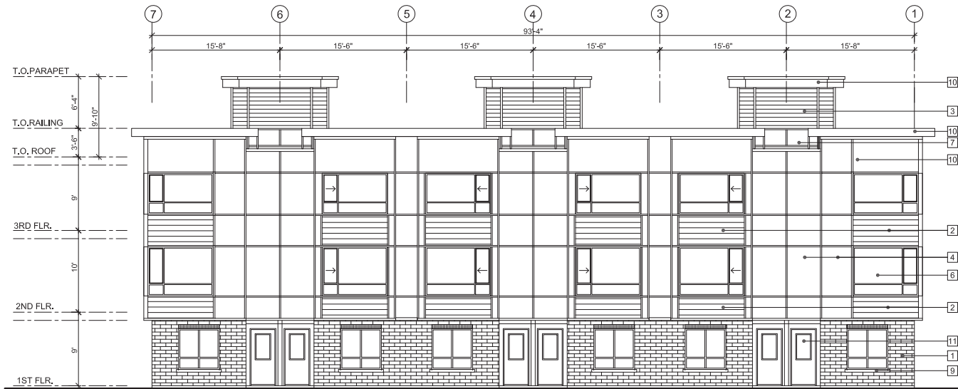
NORTH ELEVATION - BLOCK 4
