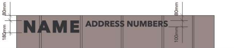
3 ADDRESS SIGN DETAIL Scale: 1:10
